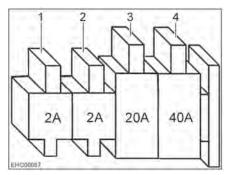
Fig. 86 Fuses for two living area batteries
