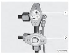
Fig. 91 Gas isolator taps position (example)
