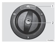
Fig. 104 Cap for the drinking water filler neck
