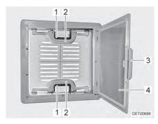
Fig. 28 Skylight with snap latch
