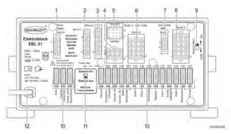
Fig. 76 Transformer/rectifier (EBL 31)
