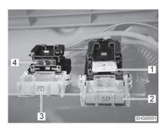
Fig. 84 Fuses on the living area battery with charging booster
