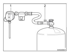
Fig. 9 Gas regulator (MonoControl)
