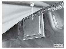
Fig. 56 Push button for electrical release
