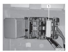
Fig. 87 Fuse on B column, right-hand side of vehicle
