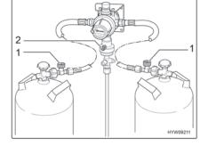
Fig. 7 Gas regulator (MonoControl)
