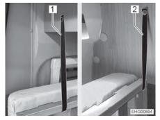
Fig. 47 Retaining straps for left-hand bed
