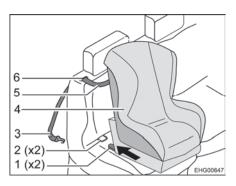
Fig. 15 Fastening with top tether
