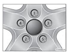
Fig. 127 Tightening the wheel nuts or wheel bolts cross-wise
