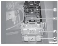
Fig. 82 Fuses on the starter battery with charging booster
