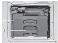
Fig. 117 Flap for the sewage tank
