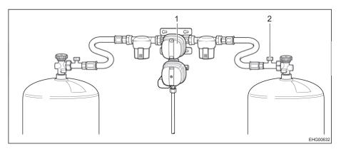
Fig. 10 Gas regulator (DuoControl)
