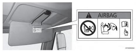
Fig. 11 Warning notice on child restraint system (front passenger's seat sun visor)
