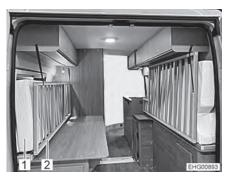
Fig. 46 Mattresses and bed bases transport position
