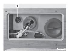
Fig. 107 Water tank with rotary handle
