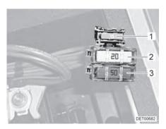
Fuses on the starter battery Fig. 81 without charging booster
