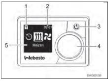
Fig. 95 Operating unit (independent vehicle heater)
