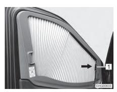
Fig. 26 Side window with folding blind
