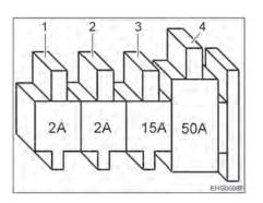
Fig. 83 Fuses on the starter battery
