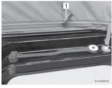
Fig. 64 Goose neck lamp, transport position
