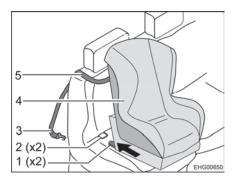
Fig. 13 Fastening with top tether
