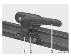
Fig. 18 Catch lever in "closed" position
