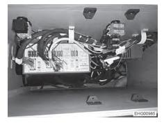
Fig. 74 Transformer/rectifier position (Fiat/Citroën)
