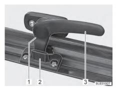
Fig. 20 Catch lever in "continuous ventilation" position
