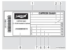
Fig. 125 Vehicle identification plate
