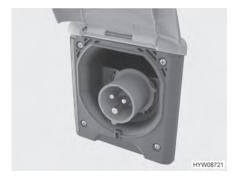
Fig. 79 230 V connection on the vehicle (CEE socket outlet)
