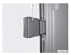
Fig. 37 Sliding window without lock
