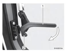
Fig. 41 Catch lever, on the side ("open" position)
