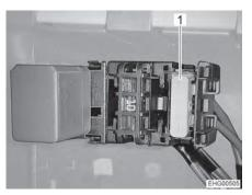
Fig. 113 Fuse on B column, right-hand side of vehicle
