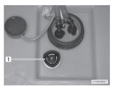
Fig. 139 Water tank with rotary handle
