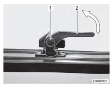
Fig. 40 Catch lever, at the bottom ("closed" position)
