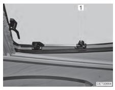
Fig. 47 Roof window with rotary hinges, open
