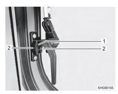
Fig. 43 Catch lever, on the side ("continuous ventilation" position)
