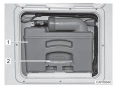
Fig. 157 Flap for the sewage tank
