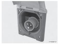
Fig. 103 230 V connection on the vehicle (CEE socket outlet)
