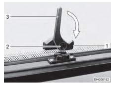
Fig. 42 Catch lever, at the bottom ("open" position)
