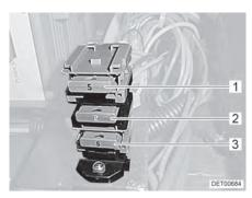
Fig. 110 Fuses next to transformer/rectifier (Fiat/Citroën)
