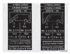
Fig. 173 Tyre pressure information sticker on B column (example)
