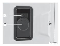
Fig. 32 Door lock (conversion door, inside)
