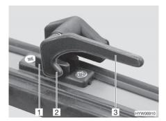
Fig. 46 Catch lever in "closed" posi-
