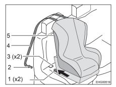
Fig. 15 Fastening with top tether
