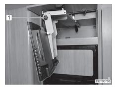
Fig. 67 Flat screen in television position
