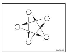
Fig. 171 Tighten the wheel nuts or wheel bolts cross-wise
