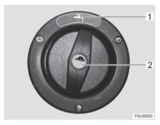
Fig. 136 Cap for the drinking water filler neck
