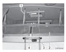
Fig. 77 Access ladder and safety net
