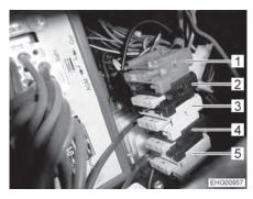
Fig. 111 Fuses next to transformer/rectifier (Ford)
