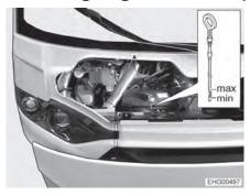
Fig. 12 Oil dipstick (engine oil)
