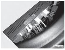
Fig. 99 Transformer/rectifier position (Ford)
