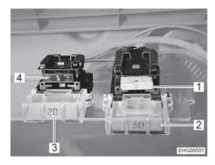
Fig. 108 Fuses on the living area battery with charging booster (Fiat/Citroën)
