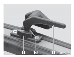
Fig. 48 Catch lever in "continuous ventilation" position
