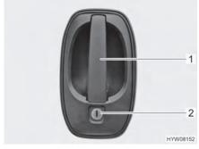
Fig. 31 Door lock (driver's door/conversion door, outside)
