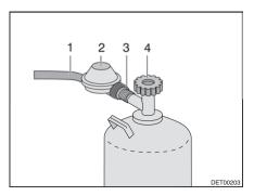
Fig. 95 Gas bottle connection
