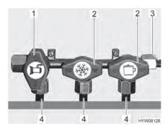
Fig. 97 Gas isolator taps position (example)
