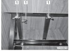
Fig. 20 Secure the attachable seat with wing nuts
